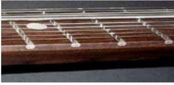
Rails are made from 3/16" stainless steel square stock, then milled along the bottom corner to a 5-sided end view, then slid from the side into the fretboard, bound by epoxy. Most of the steel is sub-surface, anchoring each Rail against any upward or sideward pressures.
